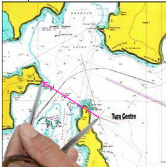
Figure 3 Measuring the Reference Point Distance from the turn centre.
